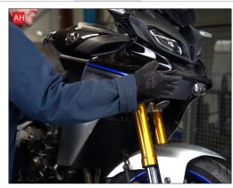
AG) Tighten the 2 upper radiator mounting bolts.
