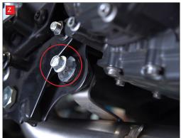
Y) Fully tighten header nuts.
